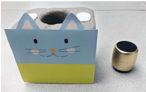
Figure 3: Portable, tangible voice agent with open top and Bluetooth speaker on the side.
